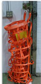
**5.** Stow by disconnecting from one side and rolling to the other. Hook the top strap to the top bracket as shown to the left.
